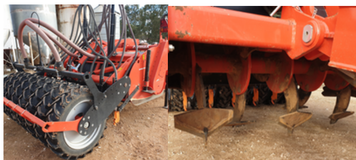
Figure 2. The trial spader worked to approximately 30 cm in heavy clay after deep ripping.
